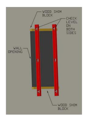
Bubbles on the builder's level must read the same for both vertical sides.
