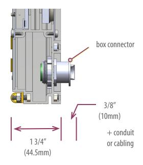
Rough opening should be <u>plumb</u>, <u>square and dimensionally accurate</u>.
