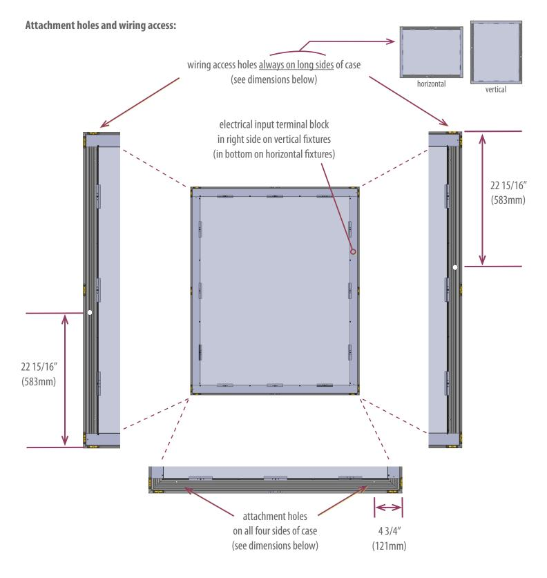
Wiring access holes — 1/2" trade size (7/8" [22.2mm] dia.), centered 1 1/6" (27mm) in from outside edge and 22 15/16" (583mm) in from end
